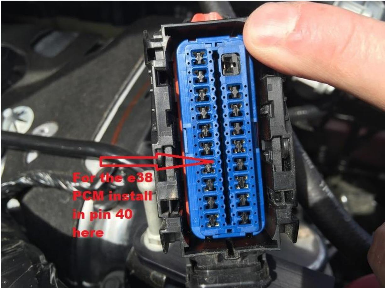
7. Find Pin location #40 as shown in the picture above. With a small pin or pick push out any plastic slug from the terminal side if hole is plugged, take the white wire and insert into the #40 pin location and seat all the way down just like the other factory terminals making sure you have the pin aligned the same way as the others. If necessary, remove the cover from the face of the plug to ensure you have fully seated the pin terminal. Then reassemble the connector.
