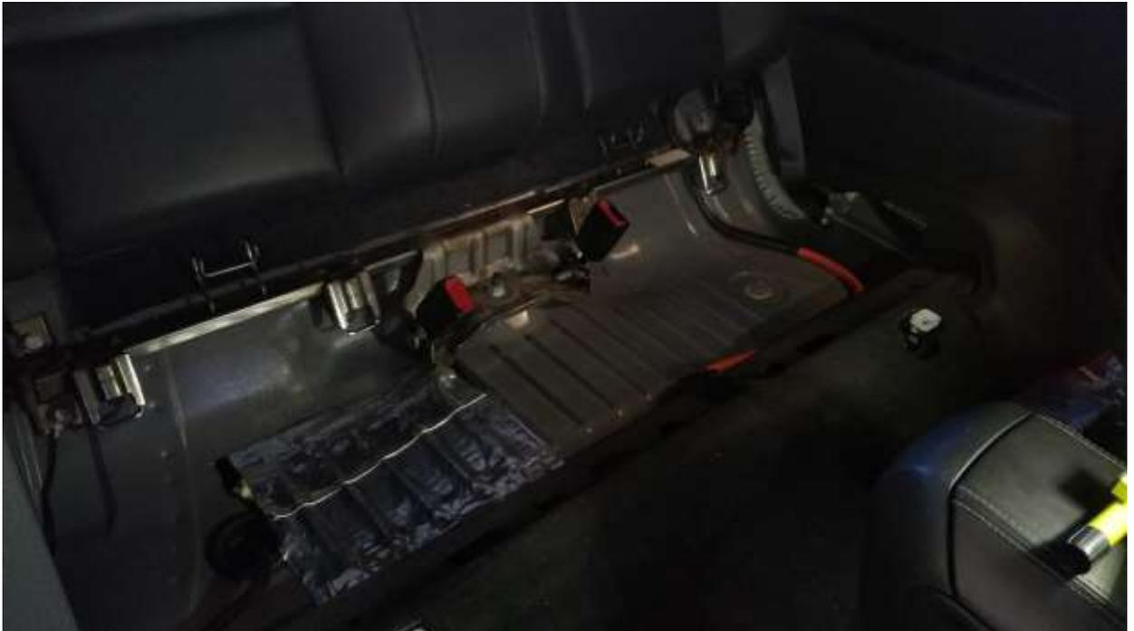
4. With the bottom section released you'll see the bracket holding the center seat belts and outer 4 bolts holding the back section. Remove the 4 15mm bolts from the sides the single 18mm nut from the center, lift the entire assembly up and remove from the car.
