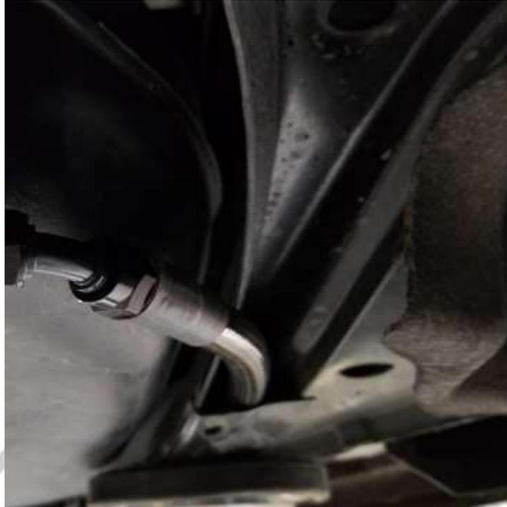
You may find that routing it from the back forward is easier so removing the entire hose from the assembly and routing the 0-degree fitting from the back forward is easier.
