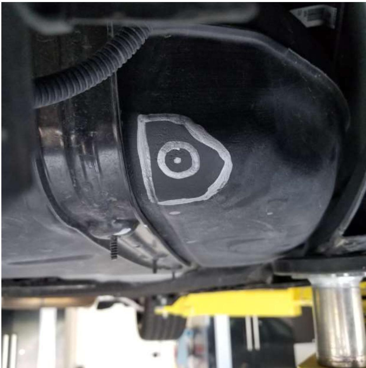
2. With the location found, clear off any dust or road debris with a shop rag and prepare to drill this location with the 37/64" drill bit mentioned on the 1<sup>st</sup> page.
