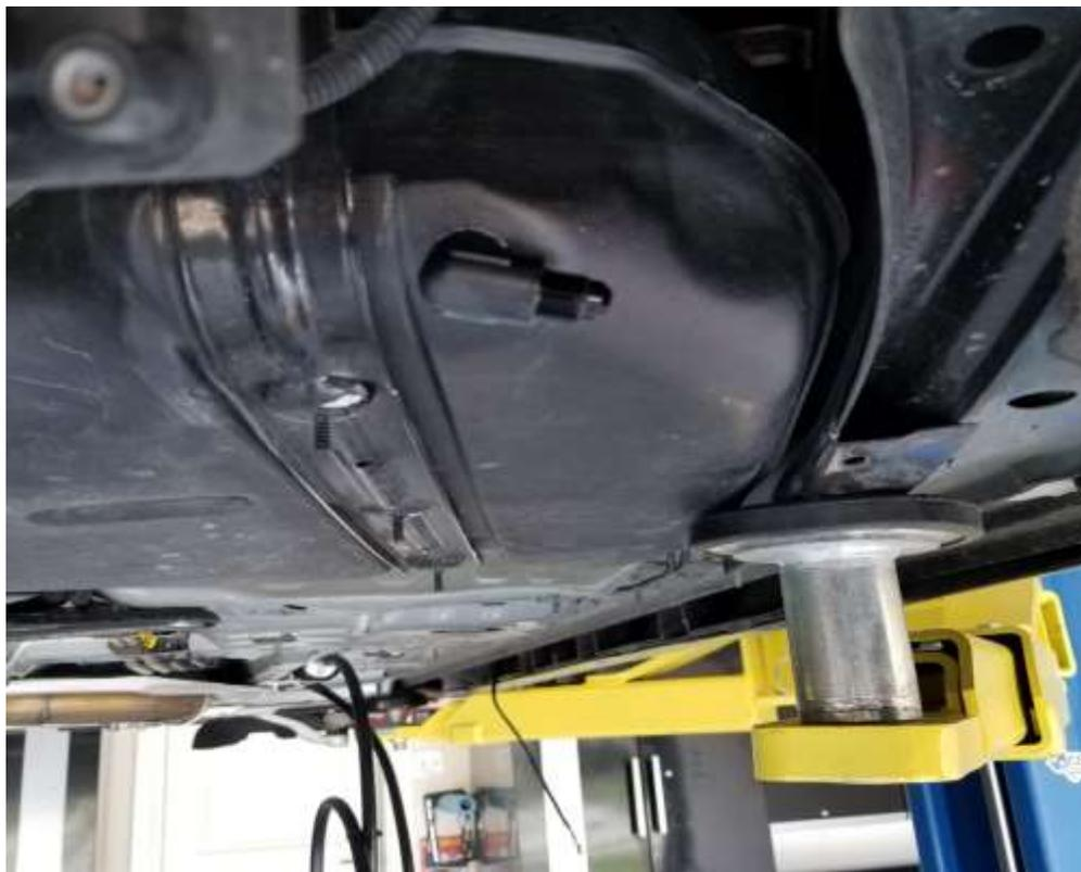
20. Now taking the other hose assembly that you just removed this fitting from, route the 45\* fitting back towards the hole we drilled in the tank, routing it through the rear brace as shown here
