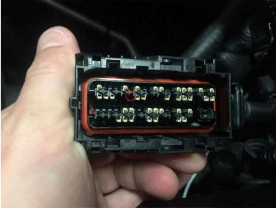
9. Reassemble harness, pug back into PCM and use remaining zip ties to secure the wires/loom out of any danger.
