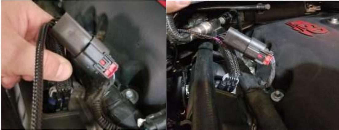
3. Route the remaining single white tipped signal wire forward towards the fuse panel, securing it safely around anything hot or likely to pinch it. Route it ultimately to the PCM.
