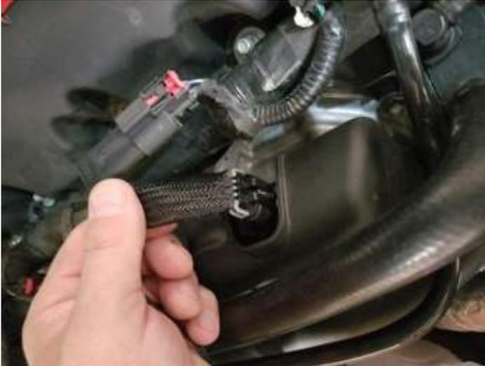
2. You will now need to gain access to the PCM located inside the passenger front fender. Turn front wheels to the far right to allow access to the screws securing the fender liner or remove the passenger front wheel/tire assembly. Remove any moldings if necessary. Loosen (but don't remove) t-bolts under hood and the one in the door jamb to allow the fender to hang loose.
