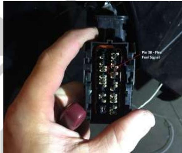
8. If there is a plastic plug in the Pin 38 location, simply pull it out with a tweezers or push it out from the front with a pick.
