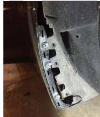
3. Once loose, you should be able to tilt the fender out enough to gain access to the PCM
