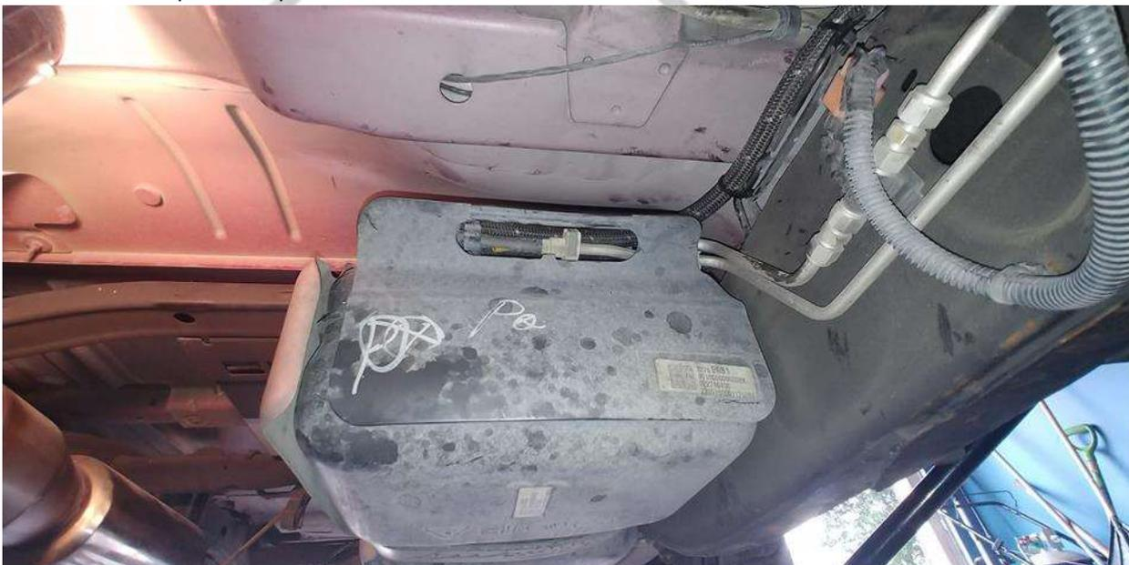
4. We'll be needing access just behind that panel, you can see in the center of the opening at the top a quick disconnect. We'll actually be tapping the feed line which is just behind the cover.
