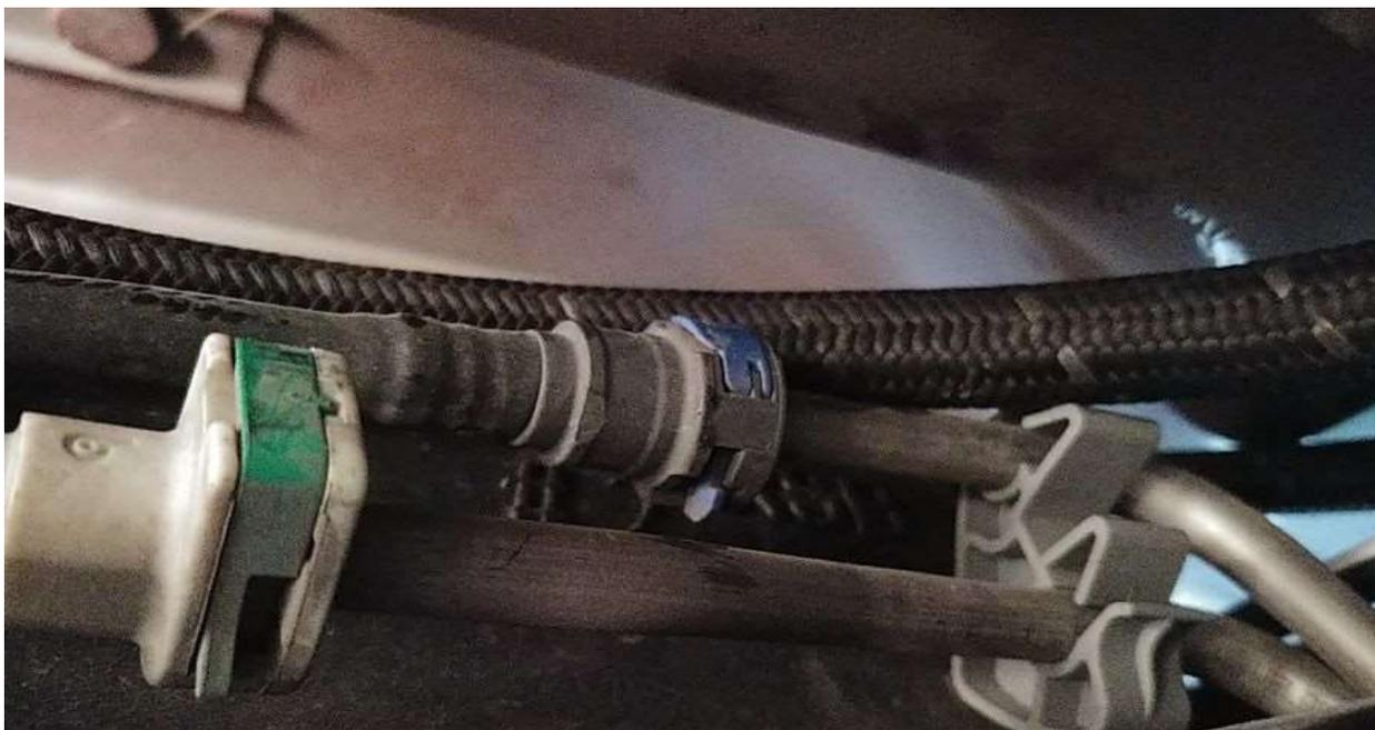
The blue clipped line is the feed to the engine we'll be with
