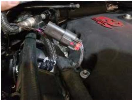
3. You should be left with one plug that can be connected to the flex sensor (if not already) and the white signal wire that will be routed to your PCM
