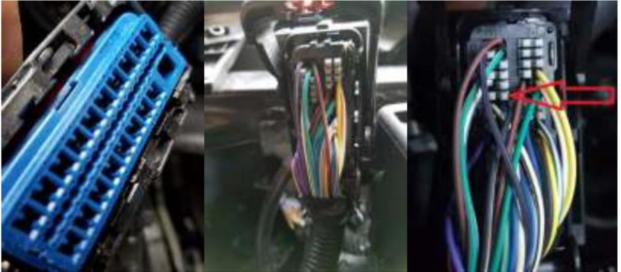
9. Once you have the absolute correct pin hole located remove the plastic plug with either a tweezers or push it out from the front with your pick if there is one and prep the hole.
