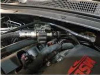
3. If you disconnected the battery like suggested above, there should be minimal fuel pressure build up, but some may spray. Have a rag ready and using the fuel disconnect tool, separate the hard and flexible lines.
