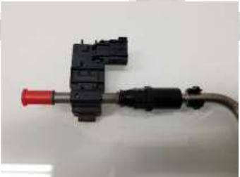
6. If your kit includes black aluminum adapters, the end cap unscrews and slides over the OEM hardline or rail. Replace the cap behind the fuel line lip and snug just hand tight using that 5/8” wrench from the tool list above (do not drop this cap as we do not have replacements readily available and charge \$10 plus shipping to send you a new one). If you have a simple flex hose, no caps come in your kit.
